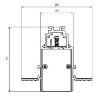
Dimensions: 1000 x 85 x 78 mm Total power: 25 w Luminaire luminous flux: 2500 lm Luminaire efficacy: 100 lm/w Weight: 1.5 kg
